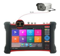
**Note:1**) If the IP camera requires PoE power, then connect the IP camera to the IP tester's LAN port . The tester will supply PoE Power for the IP camera. Click on the icon labeled POE to turn the PoE Power off or on.
