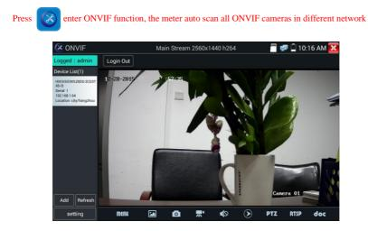
segments. It lists cameras name and IP address on the Left of screen. Tester can auto login camera and display camera image. Factory default use admin password to auto login, if you modified the password,
