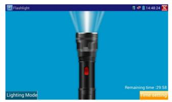
While in the flashlight app, click the red button to turn on the LED lamp. Press it again to turn it off. If you don't press the red button  $\bigotimes$  to shut off the lamp and press the button to exit the app, the lamp will stay on. Click the Time Setting button to set a timer that will shut off the lamp.
