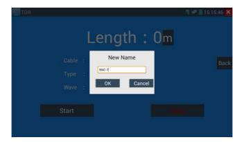
**Application:** TDR test is used for pulse reflection method, to transmit pulse signal for tested cable, when cable is open circuit or short-circuit, reflected pulse is generated, the tester receives and deals with the reflected wave, measurement results displayed on the screen. TDR can test cable open circuit and short circuit, help engineer quickly find the cable's problem location. It is more convenient and efficient to repair the faulty cable.
