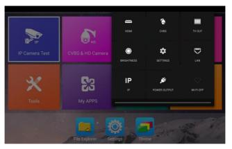
**HDMI**: Click HDMI IN to enter, in HDMI IN mode, it can converter test from analog to digital with dual test window IP & HDMI IN or Analog & HDMI in
