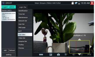
When the image is enlarged, if not operate on touch screen, it can operate by the keyboard, press the key  $(\overline{TEE^+})$  to zoom in , press the key  $(\overline{MDE^-})$  to zoom out , press upward and downward key to move image.
