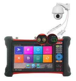
(1) Connect the SDI camera's video output to the IP tester's "SDI IN" interface, the image will display on the tester. The tester only come with SDI input interface. There is no SDI output interface.
