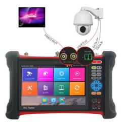
(1) Connect the camera's video output to the IP tester's VIDEO IN. The image will display on the tester after pushing the PTZ icon.
