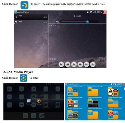
The Media player can browse video and image files. It supports the video formats of MP4, H.264, MPEG4 and MKV. The IP tester recorded files can play directly via the Media player. The Media player will automatically display the video files from the SD card. Click on the desired file to play. Click RETURN to exit.
